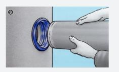
Centre the end of the pipe and push it into the seal, so that the pipe end is flush with the inner wall.
