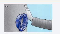
Press the F-910 seal into the hole. Do not use lubricant.
